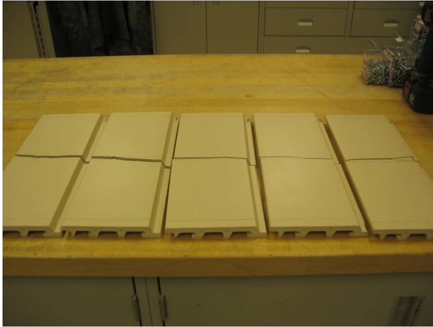
Photo No. 3 Modulus of Rupture Planes of Failure
