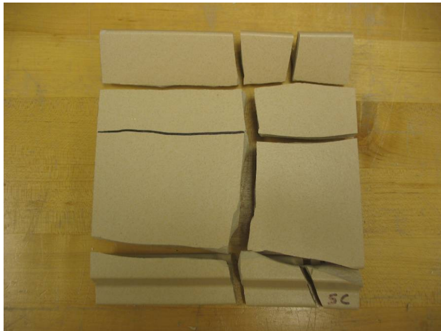
Photo No. 6 Compressive Strength Same Test Specimen Separated at Cracks
