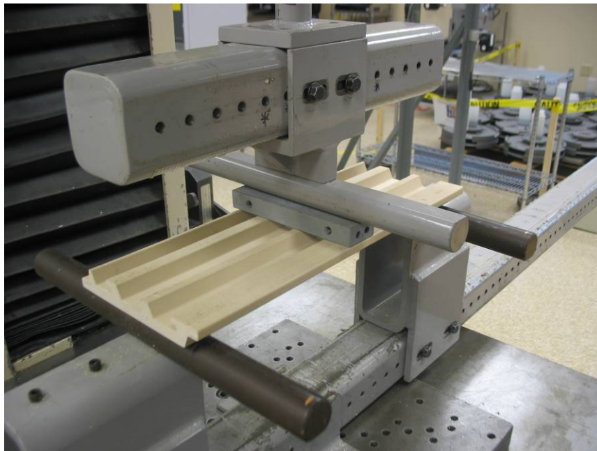
Photo No. 2 Modulus of Rupture Typical Set Up of Test
